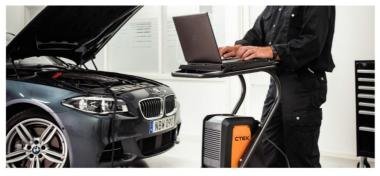
"And don't forget that ECU reprogramming and fault code diagnostics need to be carried out with the engine switched off, and the ignition switch on," Robert explained.
